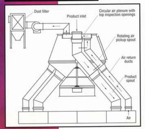
The Model E-4N Distributor allows you to vent your product bins back through the distributor to a single filter or collector. A rotating air pick-up spout rotates with the product spout to pickup air from the bin being filled. This spout is connected to the rotating, sealed air plenum. The E-4N distributor comes in the same sizes and with the same features as our Model E distributors.
